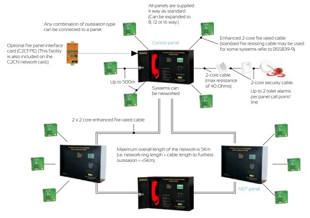
Up to 16 panels can be placed on the network (2 of these can be control panels, one of which will act as a slave unless activated as the master during an emergency).
